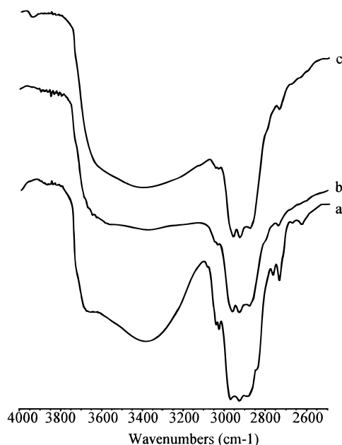
Figure 2. FTIR spectra of (a) carrier C, (b) C treated with BuLi, and (c) C treated with BuLi and CpZrCl 3 (catalyst 4).
